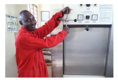
Autoclaves treat health care equipment and waste with high temperatures and steam to allow for their reuse or safe disposal. Many of the hospitals participating in the HCWH/WHO/UNDP project have installed autoclaves as an alternative to incineration.
